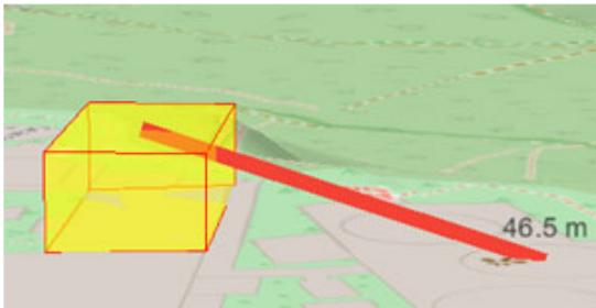
Direct euclidean distance between two points in 3D considering the terrain and the 3D objects
