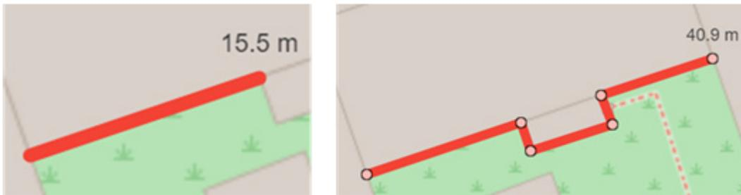
*Direct distance between two points*      *Line measurement as polyline*
