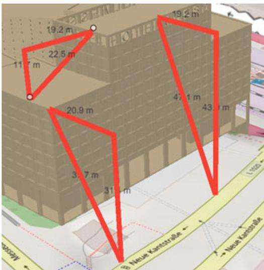
Height measurement on / with the 3D object up to the terrain
